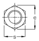
d = M10 s min d max = 10.80 Threa d min = 10.0 w e = 17.77 m1 max = 5.0
